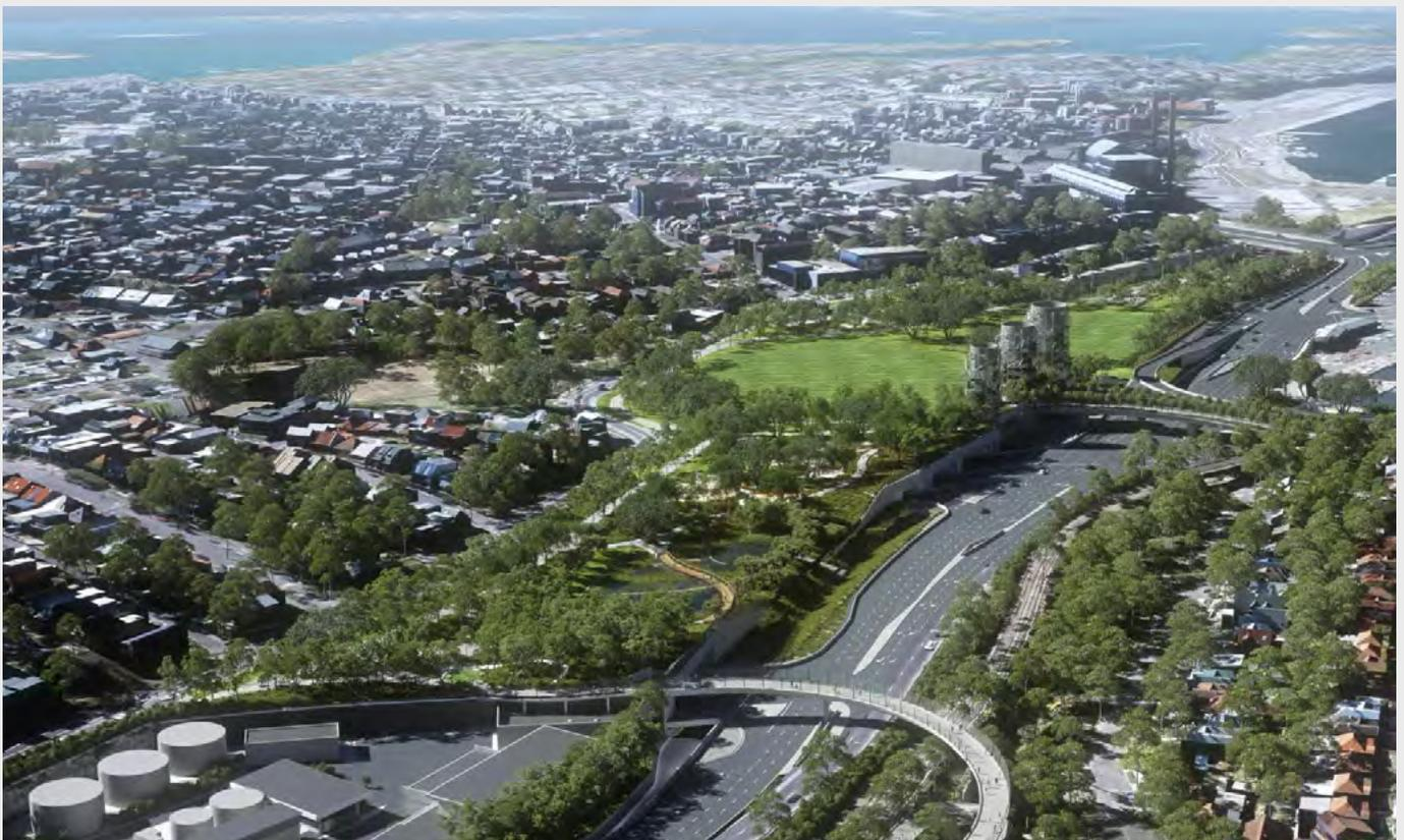
Rozelle Railyards has been an unused and derelict space for decades. As part of the WestConnex project it has been cleaned up, decontaminated and being turned into a large piece of green public open space and playing fields. The motorway tunnels are located beneath the parkland and the portals and ventilation buildings are along the City West Link frontage.
