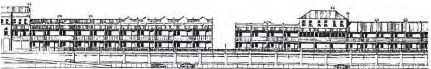
As shown in this elevation, the existing built form is considered and the motorway designed to fit into the character of Surry Hills, with the pillars of the retaining walls reflecting the design of the terraces.
