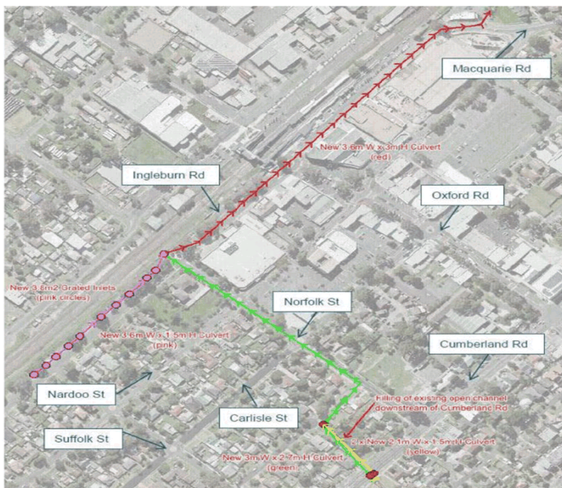
Figure 33. Layout and details of flood modification options in Ingleburn CBD
