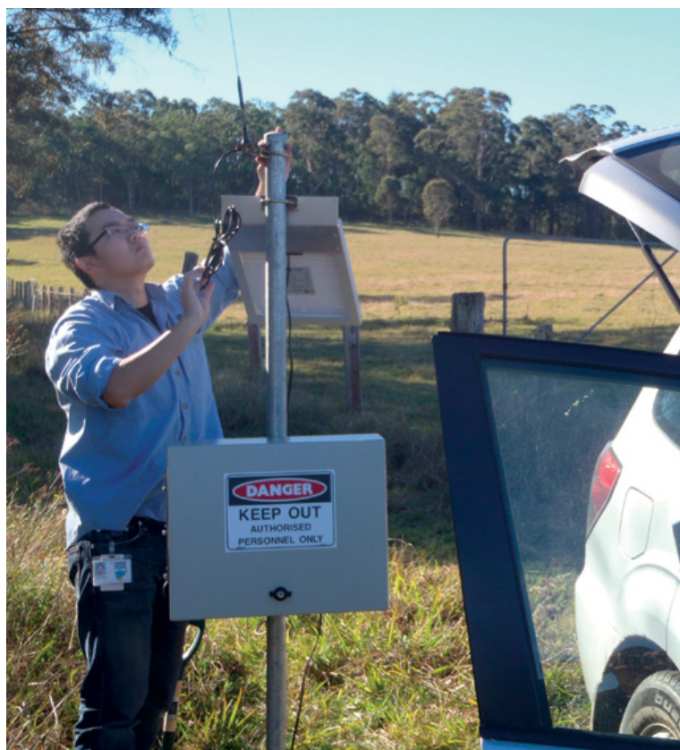
Vibration Monitor being checked
