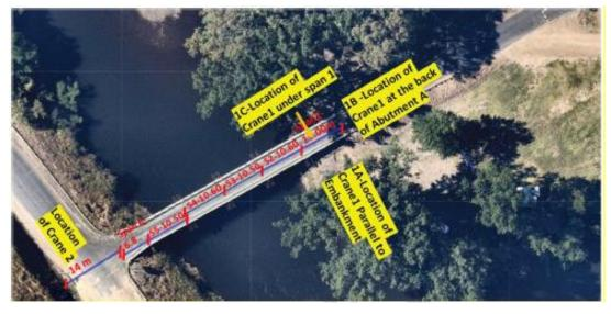
Figure 3-1: Demolition and crane work impact area
