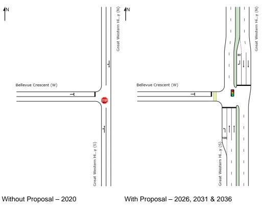
Figure 4.3: Modelled layout of the GWH and Bellevue Crescent intersection
