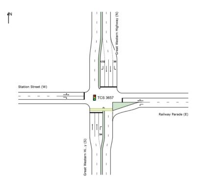
Figure 3.1: Modelled layout of the GWH and Railway Parade intersection
