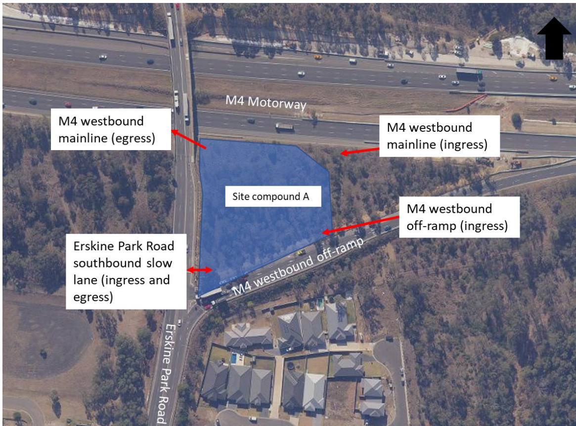
Figure 3-21 Construction Site Compound A location and proposed access points
