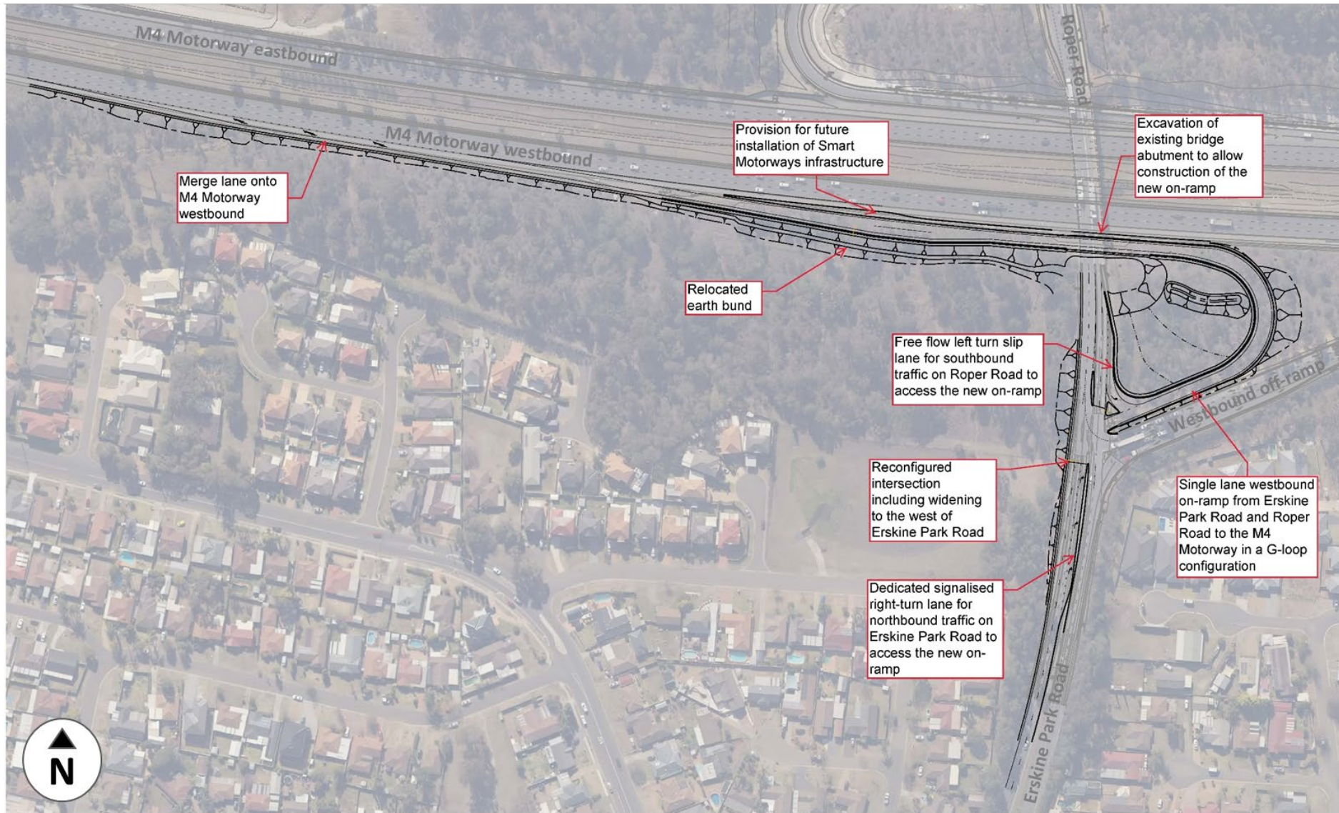
Figure 1-1 Main features of the proposal: Erskine Park Road westbound on-ramp to M4 Motorway, Erskine Park
