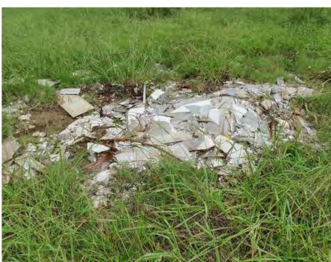
Photograph 17 – Southern Precast Site – Fly tipped fibrous boarding potential asbestos containing material (onsite)
