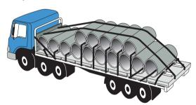
All pipes need to be clamped to prevent sideways movement.
