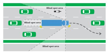
Before pulling out check mirrors, signal, check blind spot below cabin.
