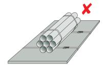
The lashings must be looped over the top to prevent rolling.
