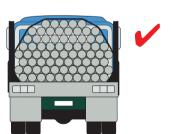
To restrain movement in loads such as pipes, they need to be crowned and have no gaps.
