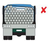
The gaps in this load can cause potentially dangerous load shift.
