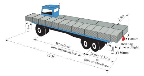
This diagram shows the allowable projected load limits.
