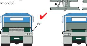
The greater the angle of the lashing to the load the greater the lashing tension will be. Angles less than 30° are not recommended.
