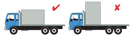
The load weight is well positioned and evenly distributed.
