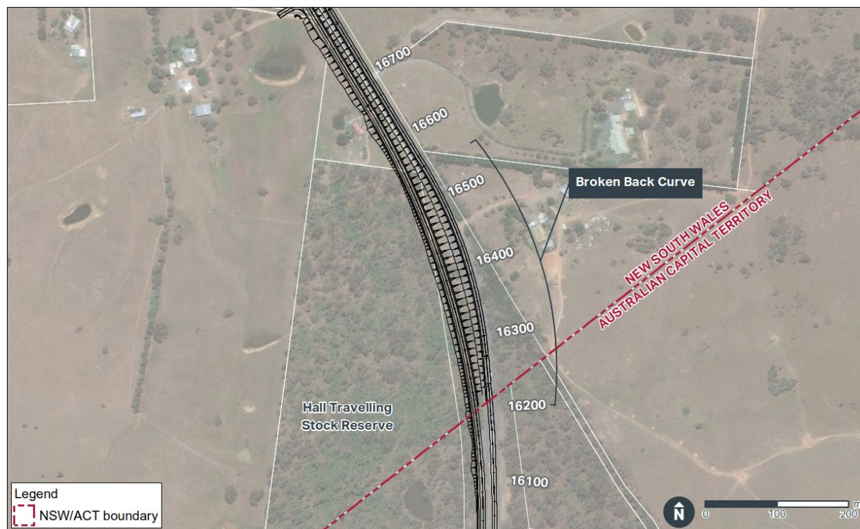
Figure 2-4 Barton highway - Broken back curve at the NSW/ACT border
