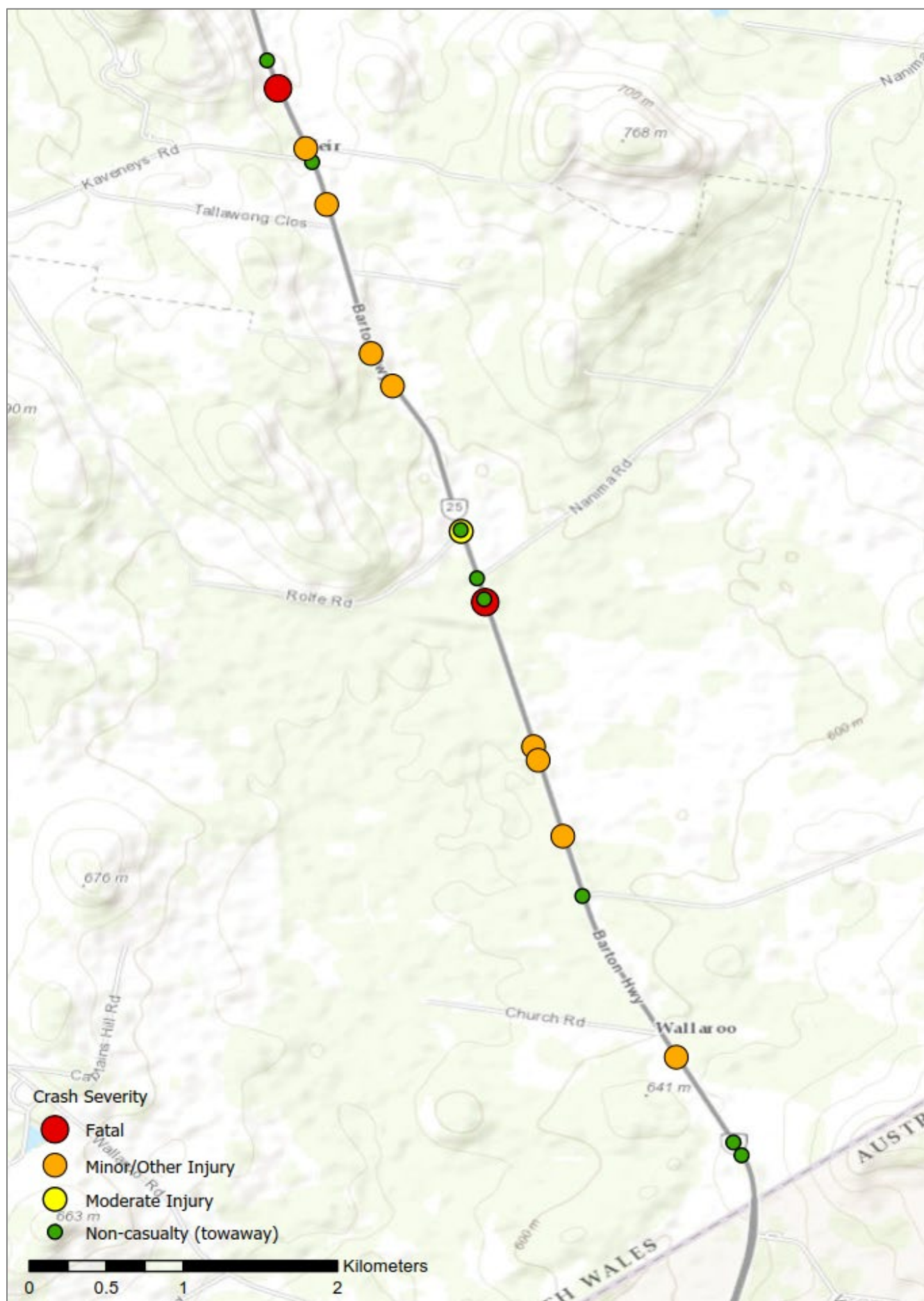
Figure 6-2 Crash plot data within construction boundary (2013-2017)
