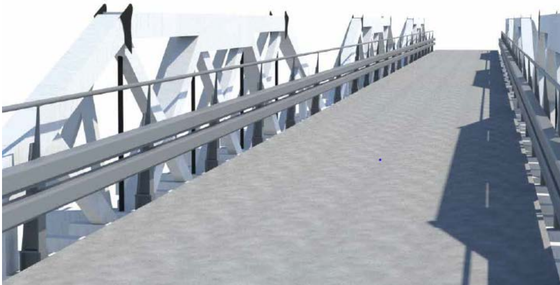
Figure 10-1 Monkerai Bridge urban design visualisation of the proposed traffic barrier railing identical to that proposed for McKanes Bridge (Source: KI Studio)
