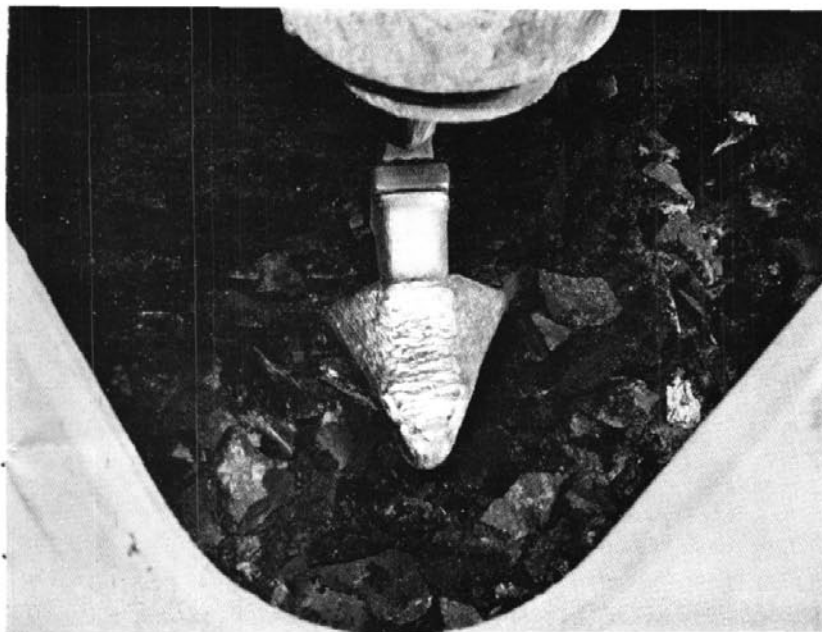
Above: The broadened ripper boot on a Cat D6 Dozer. The sharp pointed toe aids entry into the asphalt for ripping. Right: Two loaders blading loosened asphalt by working towards one another
