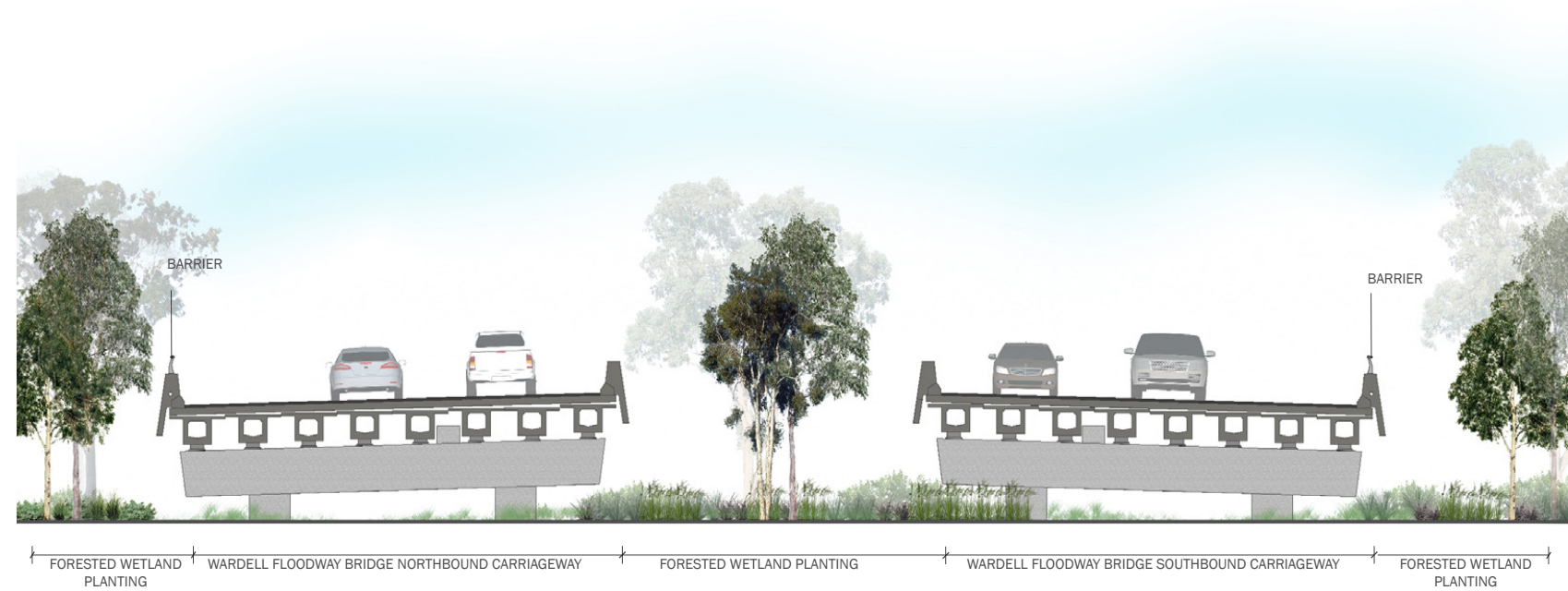
Figure 51: Typical floodway bridge (Wardell Bridge) - cross section (Scale 1:200 )
