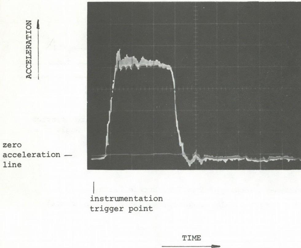
Figure 5: Typical square wave acceleration pulse obtained during the dynamic testing of buckles on the TARU sled.
