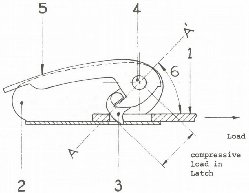
Figure 2: Compressive Latching Member Type Buckle Latch
