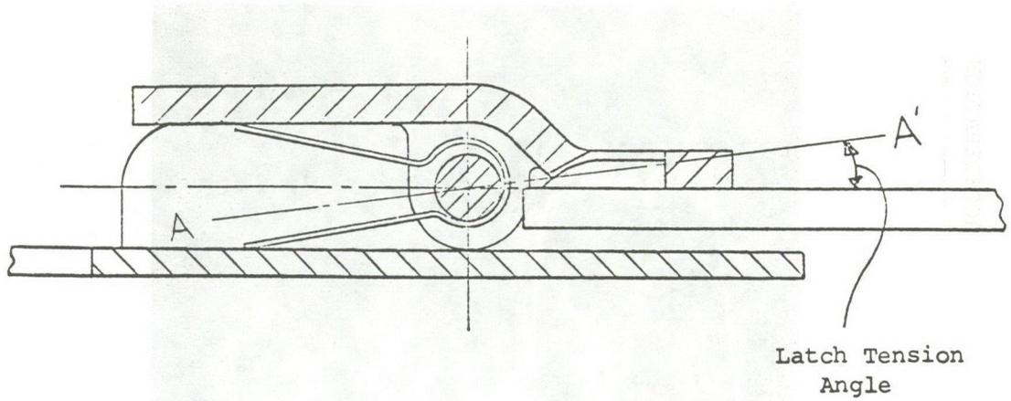
Figure 4: Tensioned Latching Member Type Buckle Latch
