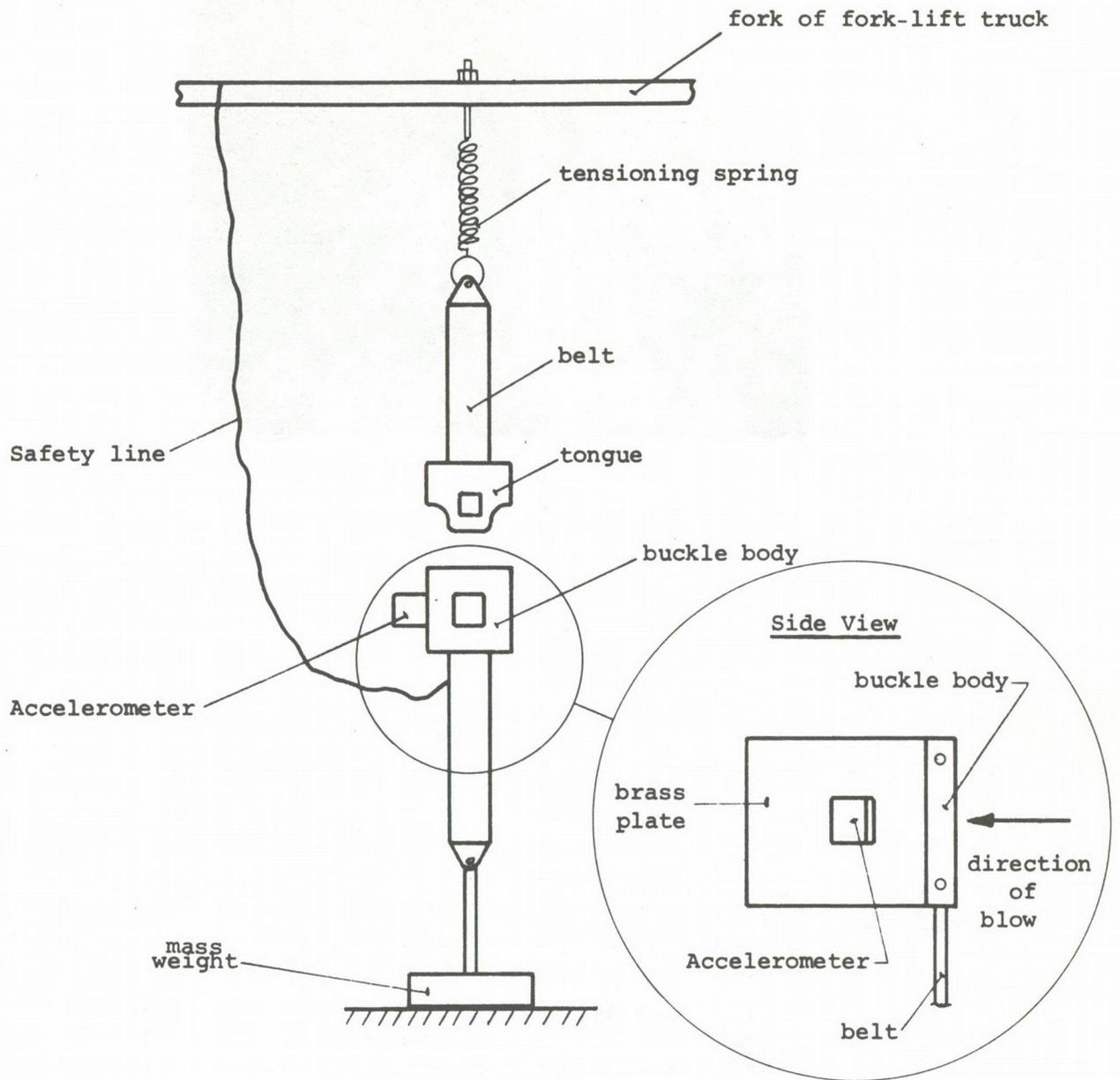
Figure 9: Schematic view of test rig used for dynamic testing of seat belt buckles subjected to high value, short duration impact pulses.
