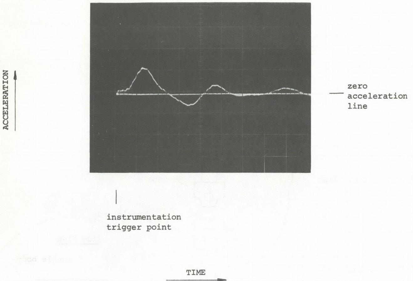
Figure 10(a): Pulse Peak of 156G, 0.32mS duration during inertial testing of buckles. Time scale, 0.2mS per division. Acceleration scale, 120G per division.
