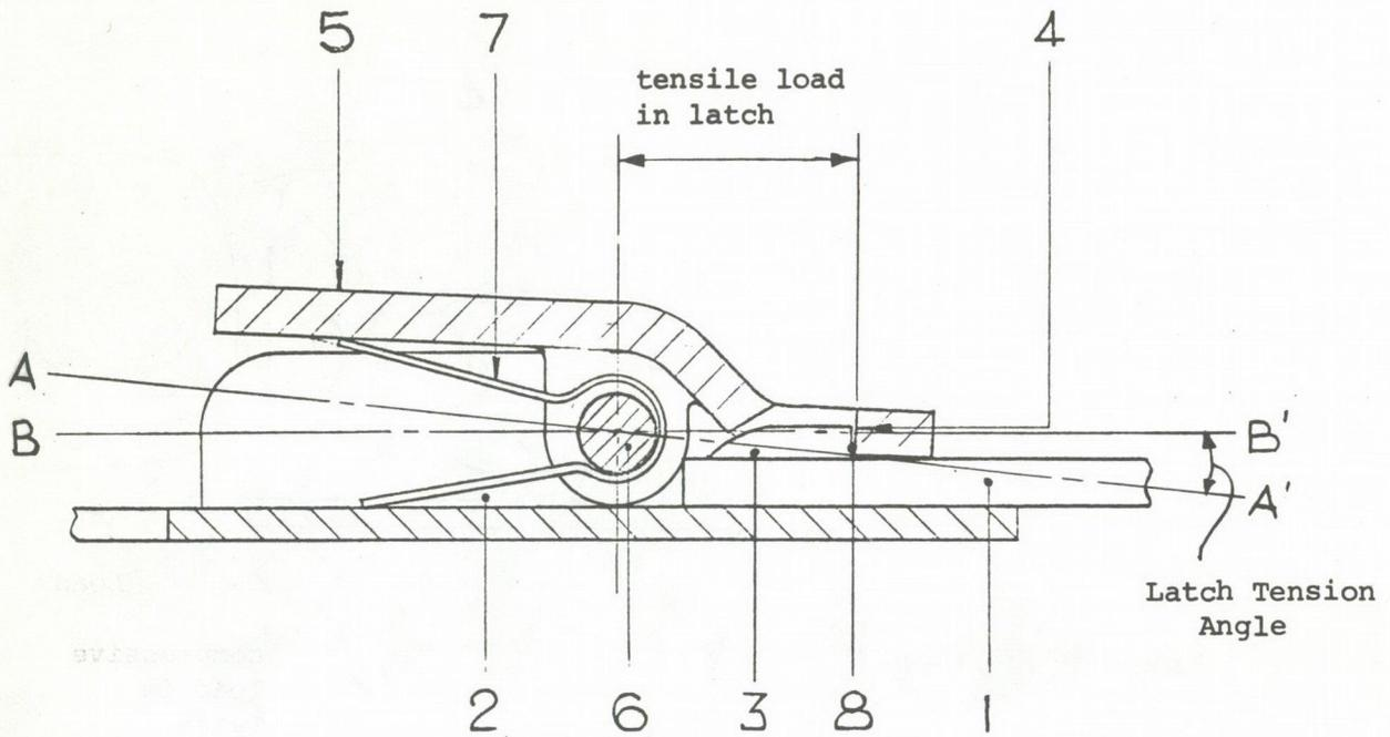
**Figure 3:** Tensioned Latching Member Type Buckle Latch
