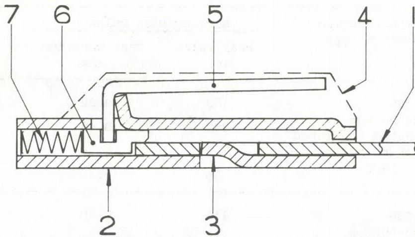
**Figure 1:** Positive Blocking Type Buckle Latch
