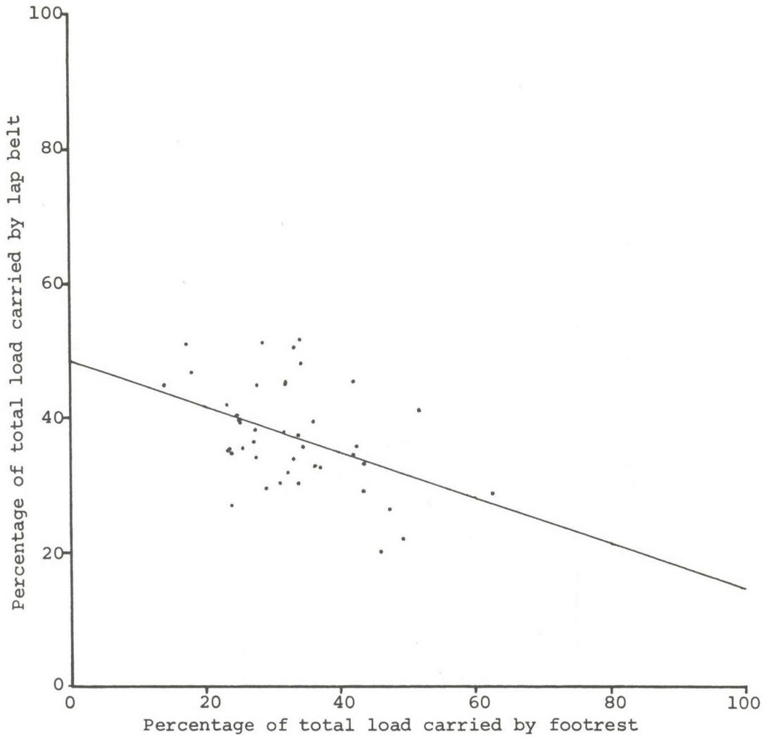
Figure 1 : Lap belt loop load (as % of total load) plotted against footrest load (as % of total load) - after Armstrong and Waters<sup>2</sup>, and Chandler and Christian<sup>3</sup>.
