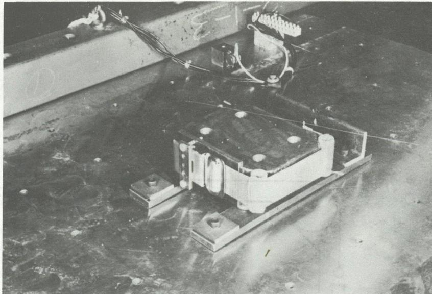
Figure 7: View of test rig used for dynamic testing of seat belt buckles (with push-button operated buckle fitted) on sled subjected to car crash accelerations.
