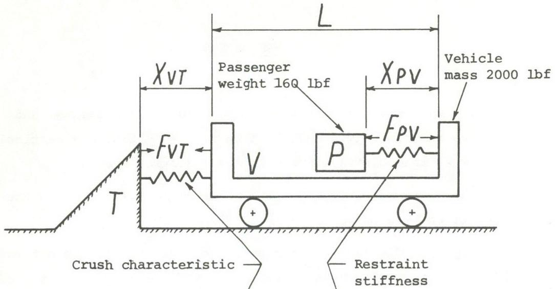
Force increases at 3000 lbf/in as vehicle presses into target
