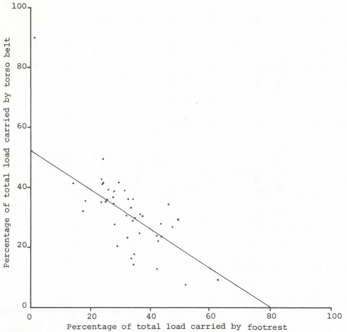
Figure 2 : Torso belt loop load (as % of total load) plotted against footrest load (as % of total load) - after Armstrong and Waters<sup>2</sup>, and Chandler and Christian<sup>3</sup>.
