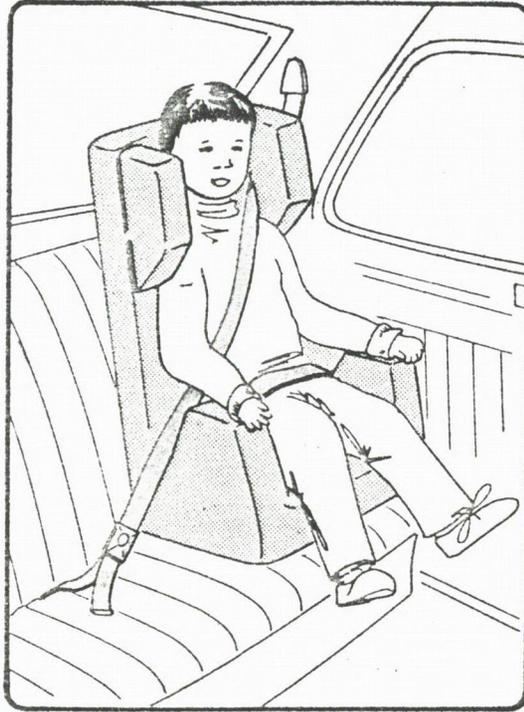
FIGURE 4: Lap-sash belt converted to child restraint by use of self-restrained booster chaise.
