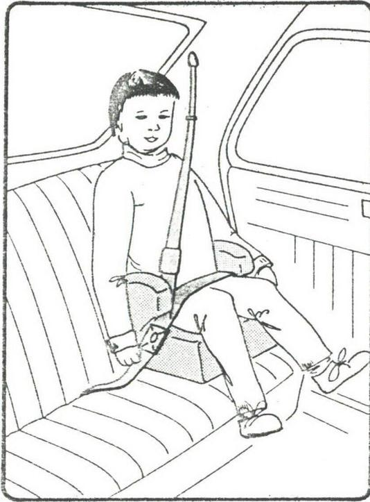
FIGURE 5: Lap-sash belt converted to child restraint by use of restrained booster cushion.
