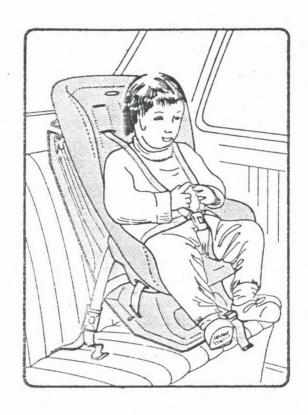
FIGURE 6: Australian "Safe-N-Sound Mark 10" forward - facing chair with harness. Central push - button release buckle with strong spring.
