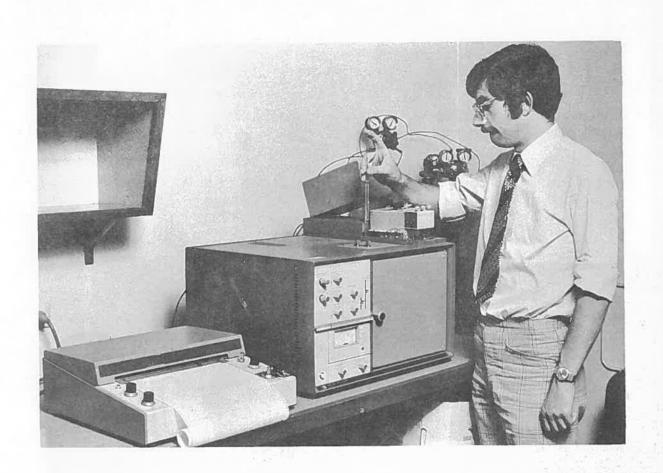
Figure 11: Gas-Liquid Chromatography - Analysis and Recording Unit.
