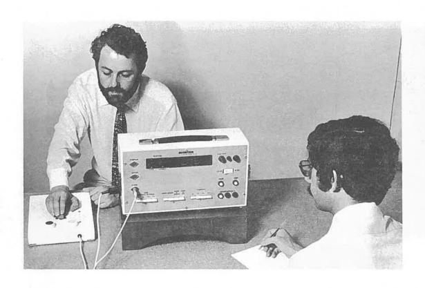
Figure 7: Reaction Time Test - Stimulus/Response and Recording Unit.
