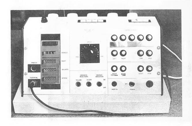
Figure 4: Motor Performance Test (Vienna Determination Apparatus)
