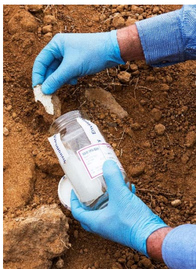
Sampling soil to find out if it is contaminated. Photo: Bottlebrush Media/EPA
