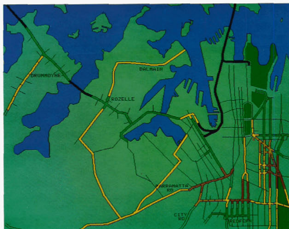
A computer graphics display wherein the principal arterial roads are colour-coded to indicate changes in current traffic densities.
