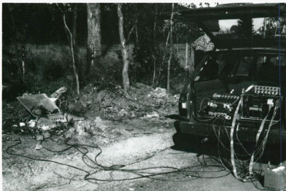
(Above) H-bar strain gauges and thermocouples are implanted below the pavement surface and connected to the Pavement Response Data Acquisition System (at right) for information recording.
