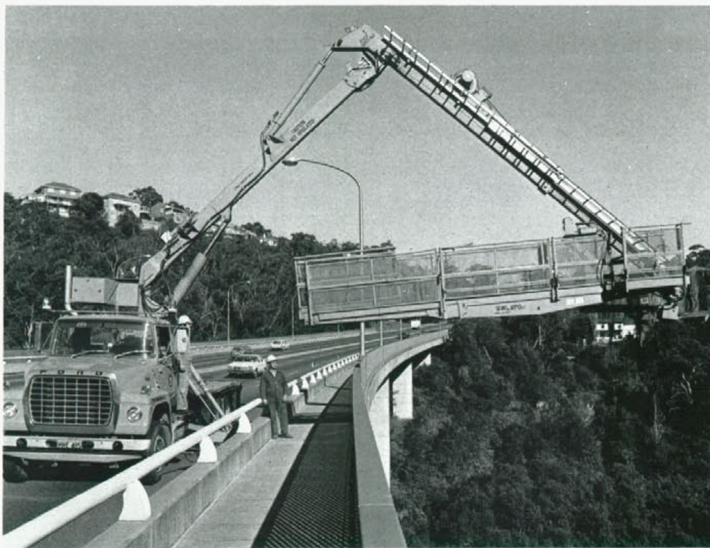
Once the wheeled outrigger is braced against the mainframe, the boom array can unfold to swing the platform over the side of the bridge.
