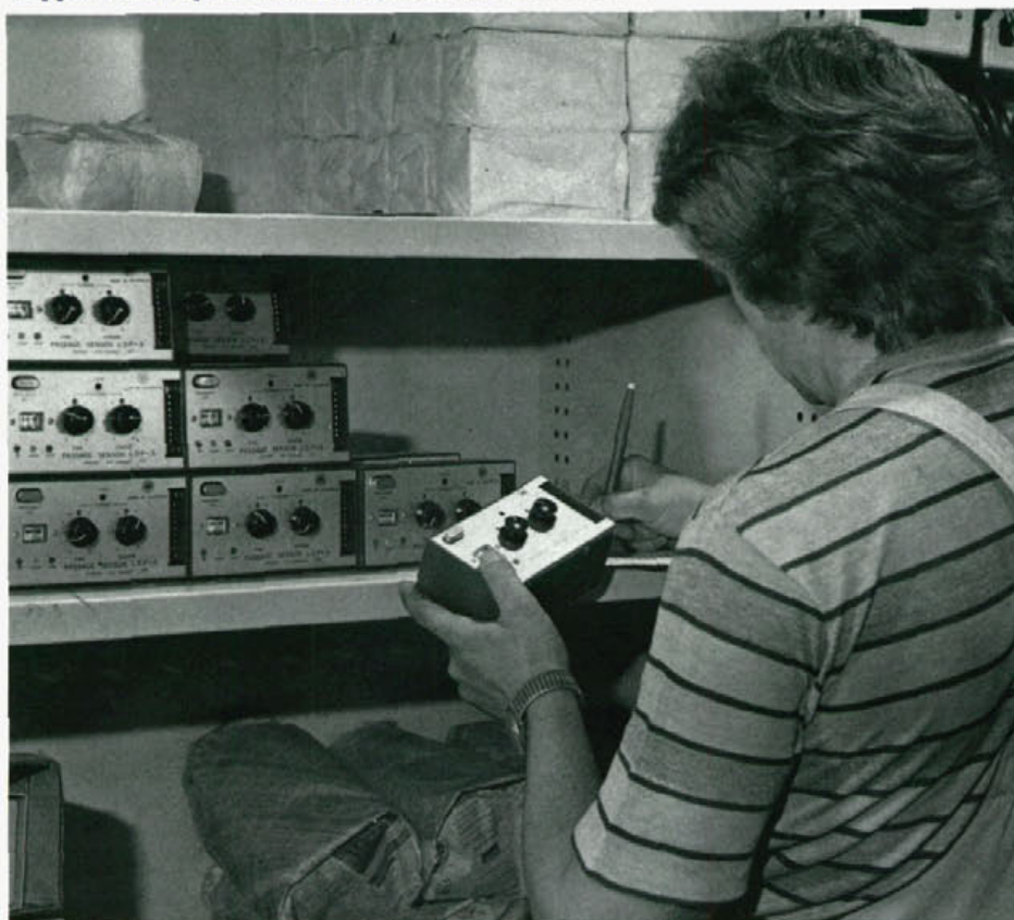
A passage sensing device used in traffic signals being taken from the stock of supplies and replacement equipment held in the store.
