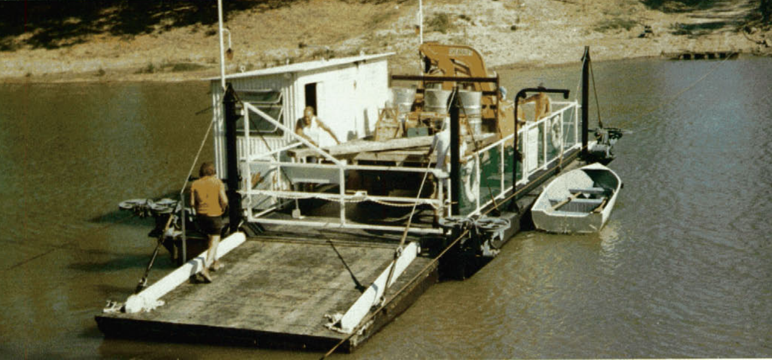
The new steel-hulled ferry on its maiden voyage with a 10-tonne test load.
