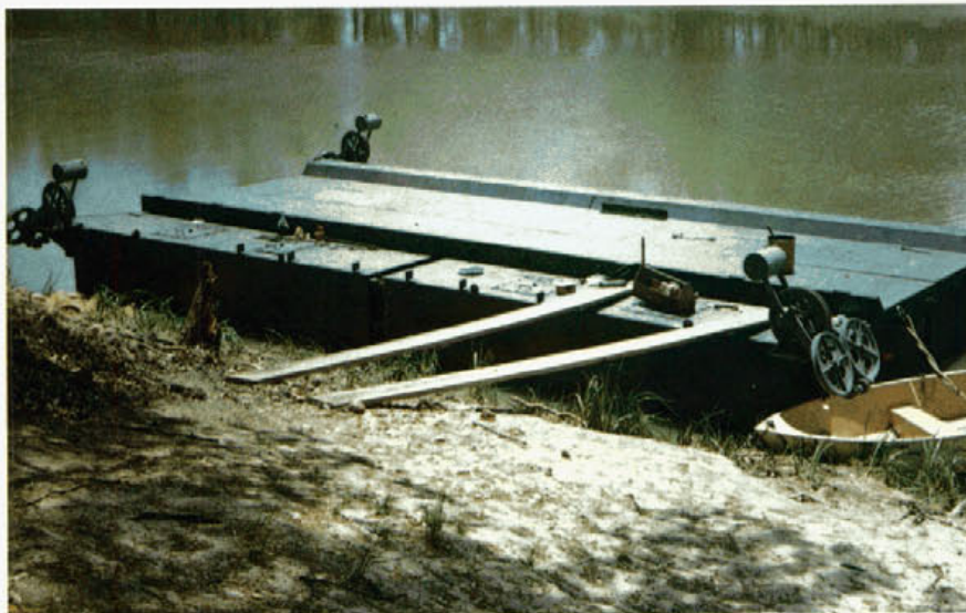
The four pontoons assembled, end guides are fitted and the ferry takes shape.
