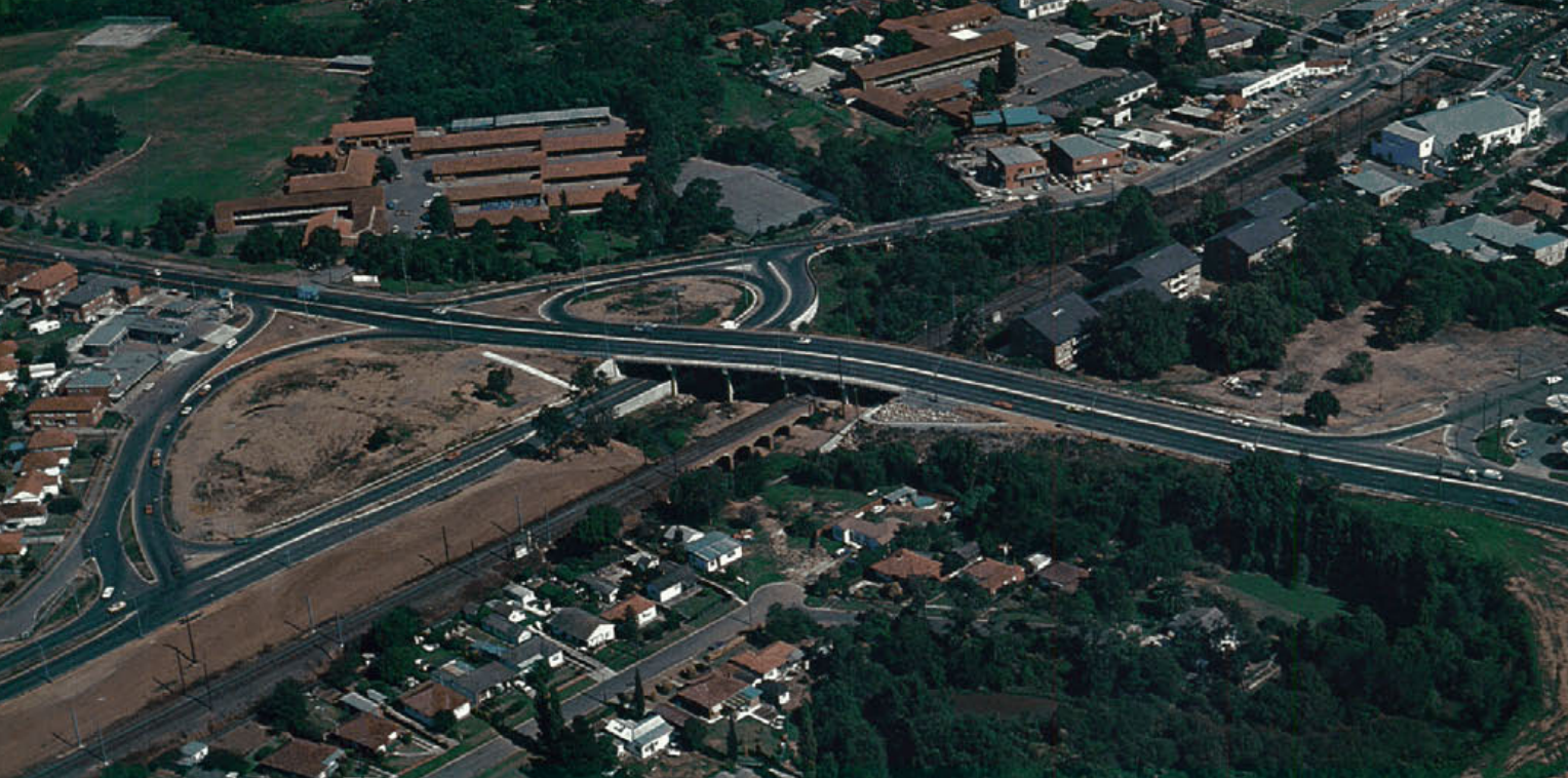
Two aerial views showing the road improvements and the extensive widening of the bridge which carries The Horsley Drive over the Main Southern Railway Line at Fairfield (see article on pages 68-69).
