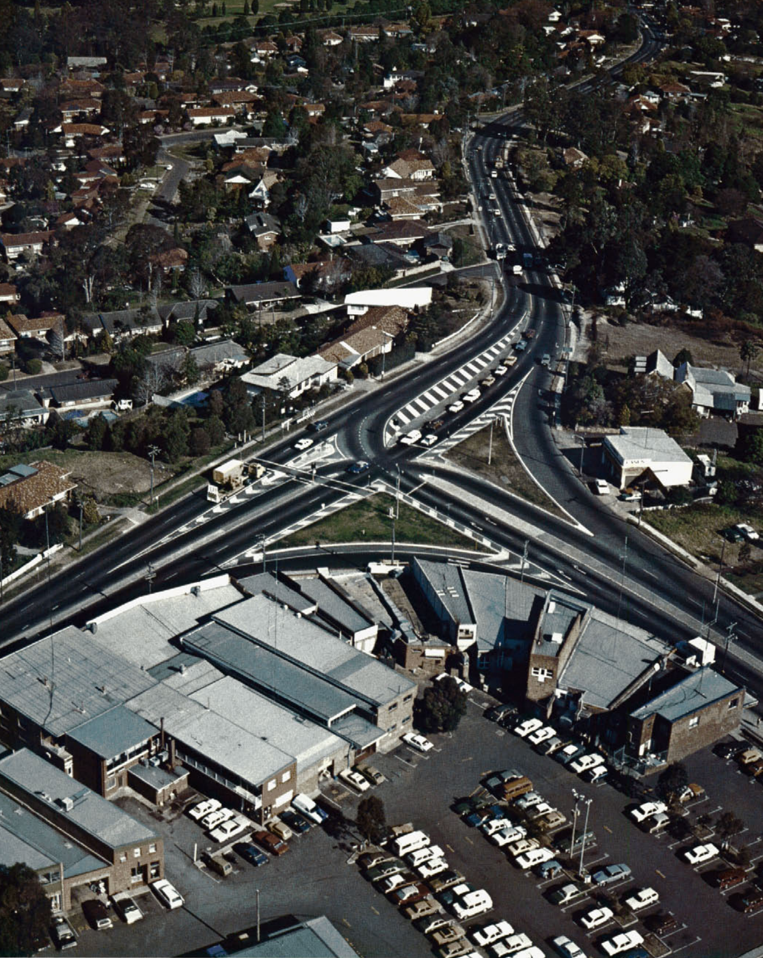
Aerial view, from above Thompsons Corner Shopping Centre at West Pennant Hills showing the junction of Castle Hill Road and Pennant Hills Road (State Highway No. 13). The introduction of traffic signals, channelisation and pavement marking has greatly improved traffic conditions at this location (see article on reliability of traffic signals commencing on page 22).
