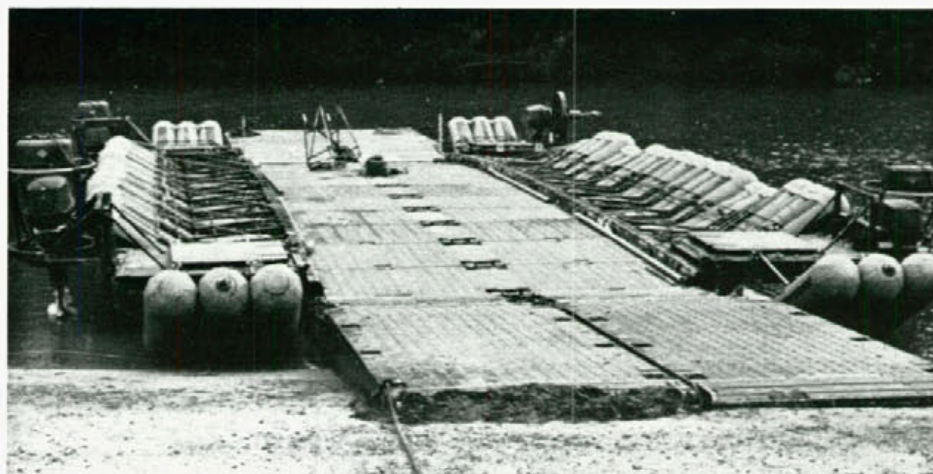
An air portable bridge constructed for use as a raft at a water crossing.
