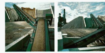
(Top): General view of the aggregate storage area consisting of twelve bins each capable of holding 2,000 tonnes of various sized aggregates and sand. The material is transferred from road vehicles by way of one or two under road hoppers and a conveyor belt system at the rate of 500 - 600 tonnes per hour.
