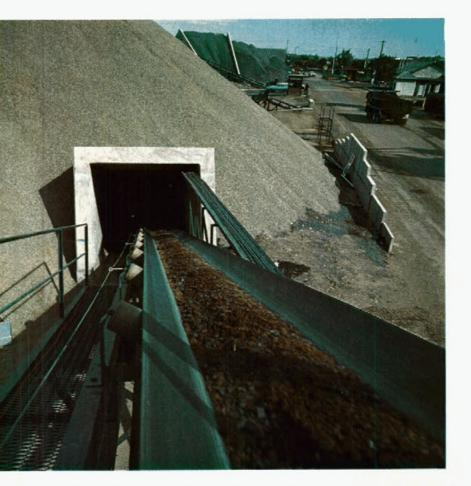
(Above): Aggregate being transferred from storage bins to the mixing plant by underground conveyor belts located in a tunnel running the full length of the aggregate storage bins.
