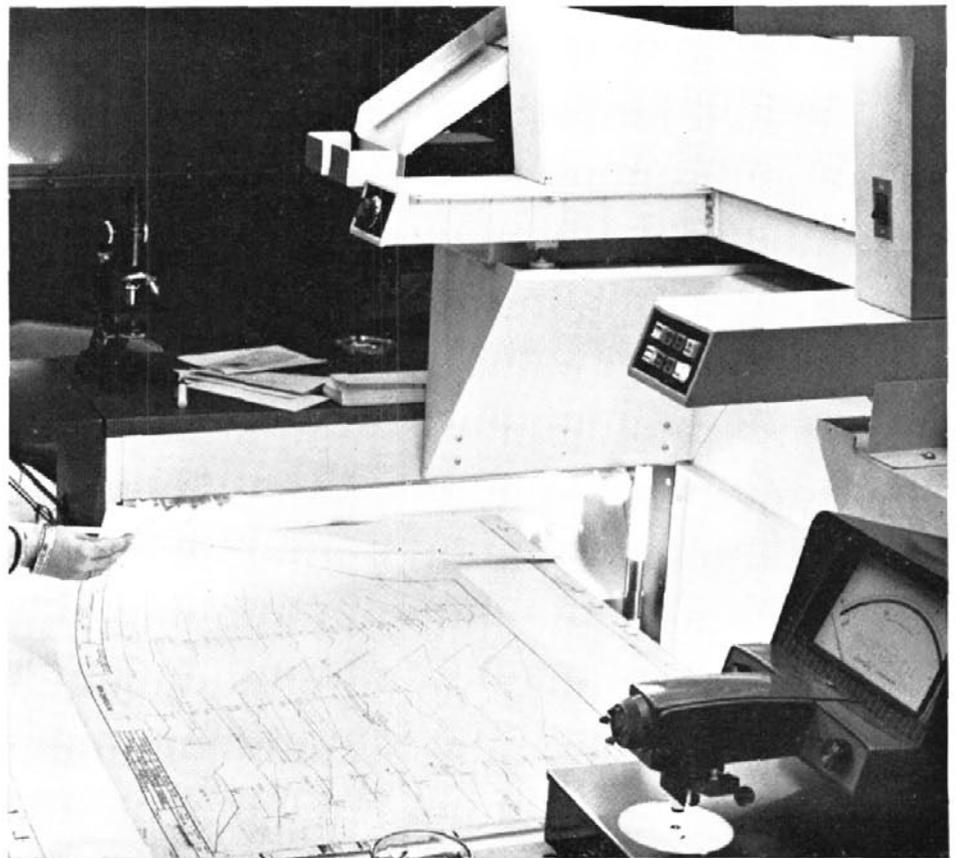
*This processor Camera is designed for use on new standardized drawings but can be also used for work where continual camera adjustment is necessary.*
