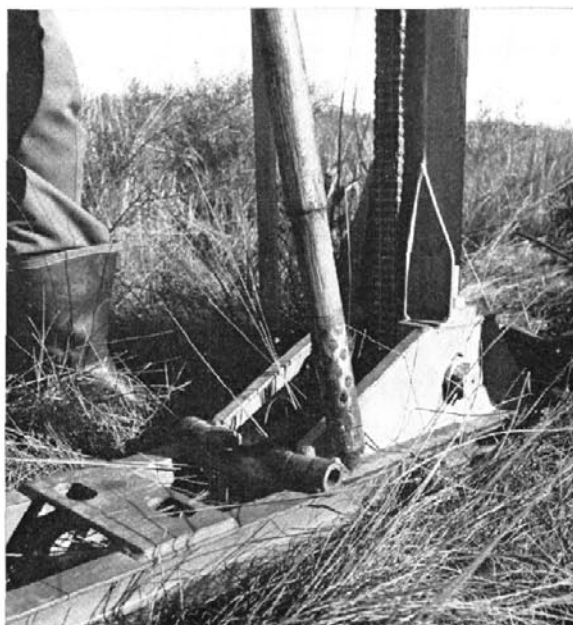
Close-up view of the tip of a piezometer
