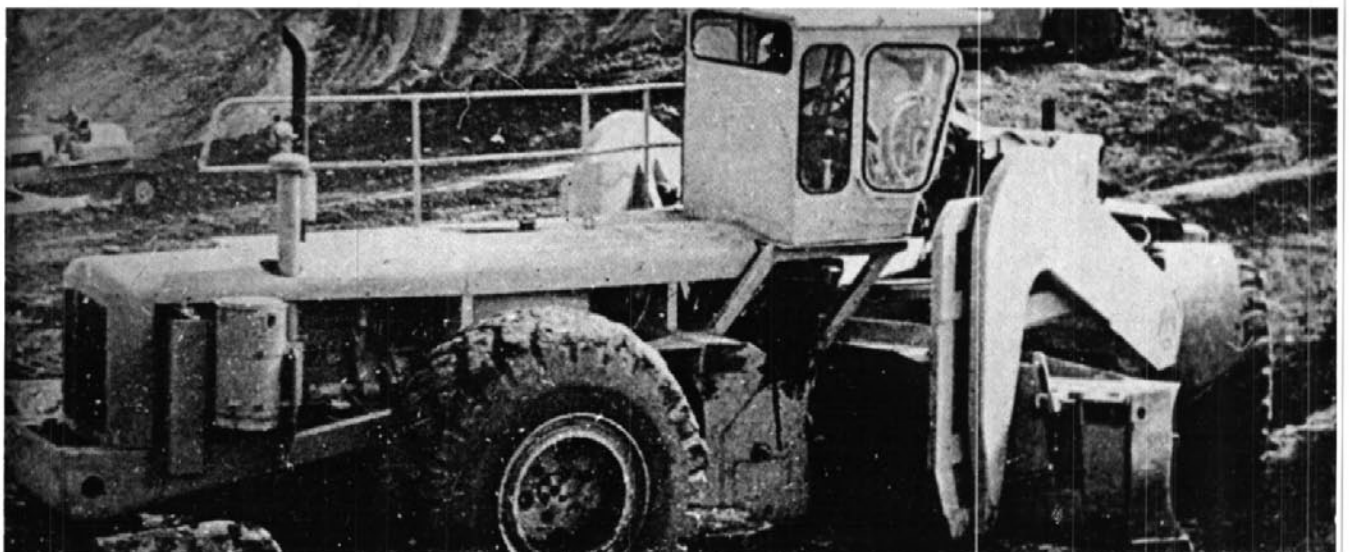
Special purpose grader of 617 h.p. and 45 tons
