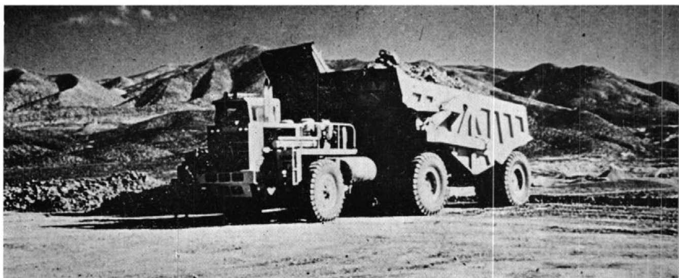
Dump truck of 79 cu yd capacity 700 h.p. engine
