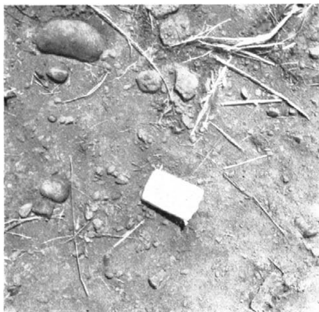
California. S.H. 41 near Fresno. Vertical close-up of natural surface prior to "oiling" and mixing.
