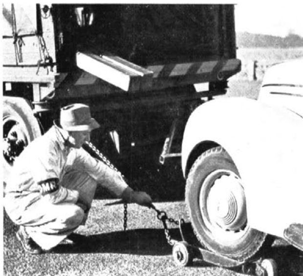
"Skate" on which wheel rests when towing cars with flat tyres.
