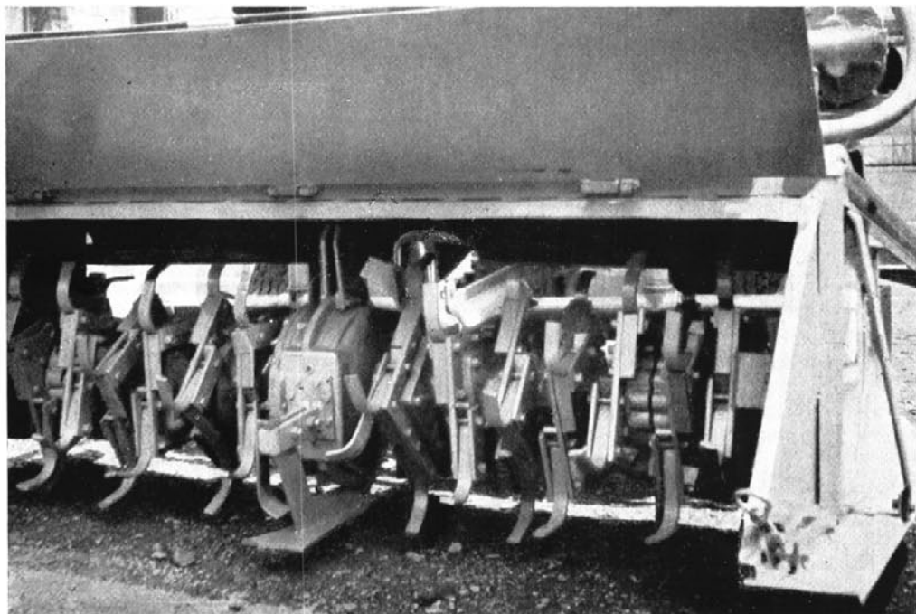
Box of roadmixing machine used for blending aggregates, mixing aggregates with bituminous binders and also for soil stabilisation.
