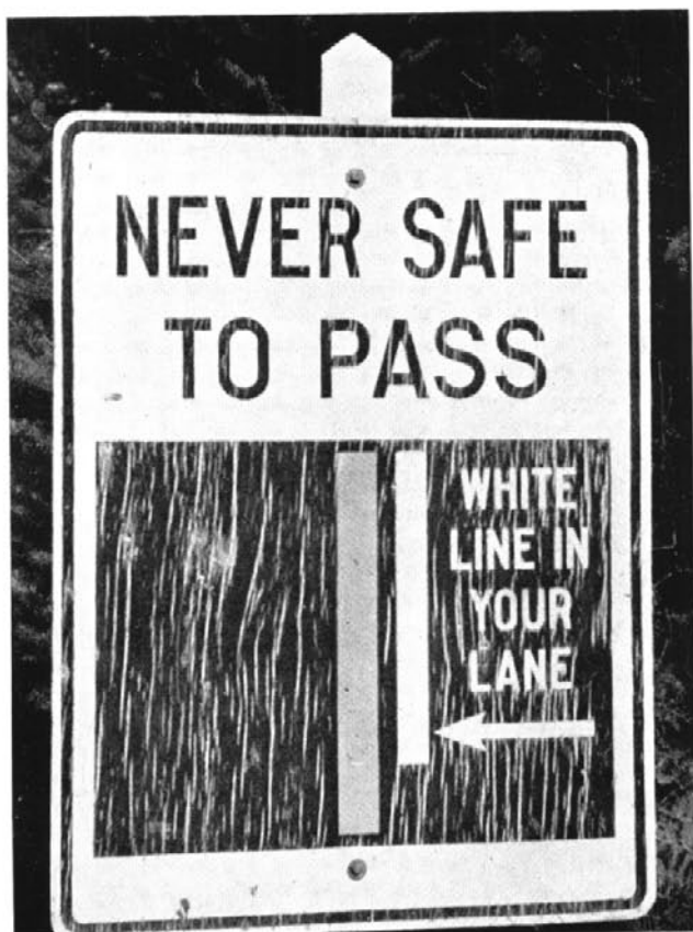
Roadside sign explaining purpose of double centre line on road where sight distance is restricted.
