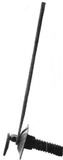
Type of Screw Jack and long handle spanner used in connection with moving of complete buildings from right-of-way. A large number of these simple jacks is used under each building.
