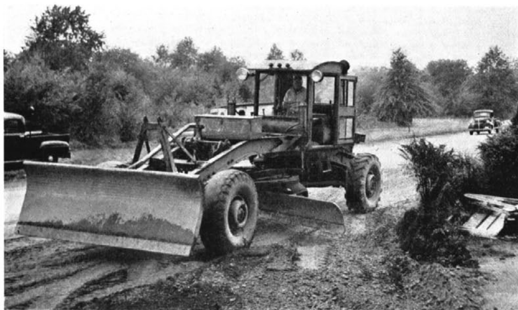
Motor grader fitted with 'dozer blade operated through scari-fier controls.
