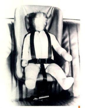
Pictured is an anthropomorhpic dummy designed and constructed in the Traffic Accident Research Unit. The dummy closely simulates a six months old child in the Unit's evaluation of infant crash restraint concepts. It has a cast aluminium "skeleton", padded with foam plastic. The spine is a steel cable assembly with nylon "vertebra". Sensors on the dummy connect to the Unit's computer to record "body" stresses under simulated crash conditions.
