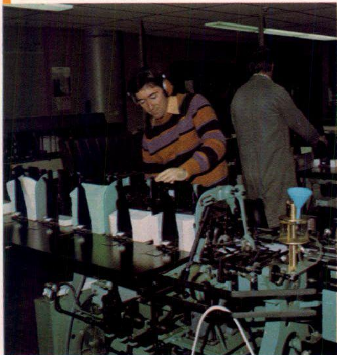
LEFT: During the year outmoded mail dispatching equipment was replaced with modern machines. The machines automatically insert material into envelopes and seal them at the rate of 5,000 an hour.
