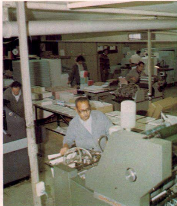
LEFT: During the year outmoded mail dispatching equipment was replaced with modern machines. The machines automatically insert material into envelopes and seal them at the rate of 5,000 an hour.
