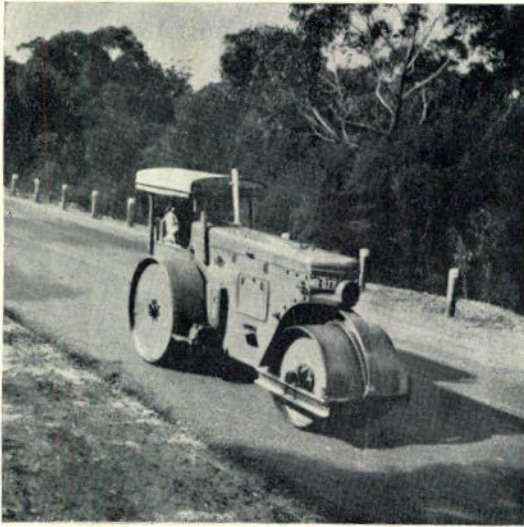
6-8 ton diesel road roller.
