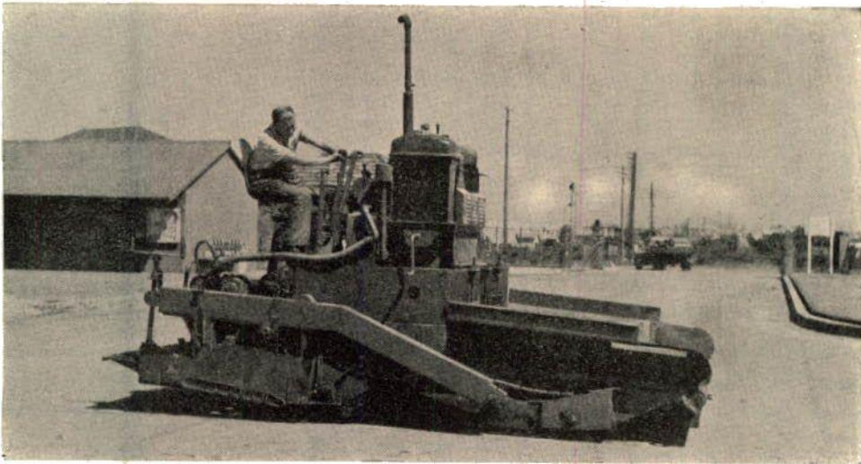
Spreading and tamping machine for bituminous pre-mixed materials.
