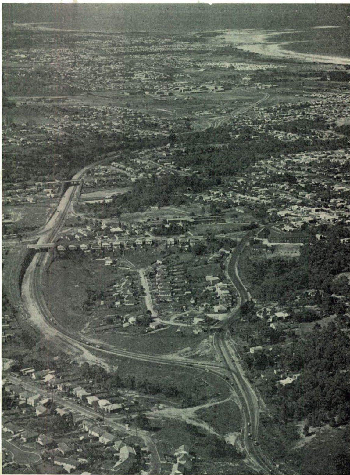
The alternative route to the Prince's Highway constructed to by-pass the shopping and business centre of Wollongong is shown on the left of the photograph. The by-pass, built to expressway standards, is two miles in length and will ultimately form part of a new north-south arterial road to be constructed from Thirroul to Dapto and beyond
