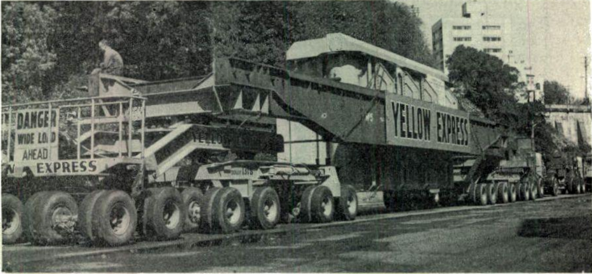
Movement of transformer weighing 180 tons from Garden Island to Cook's River railway goods yard, on a special transporter with 12 axles, 12 ft. 6 ins. wide, and 96 load-carrying tyres. It was the heaviest load to be transported by road in New South Wales
