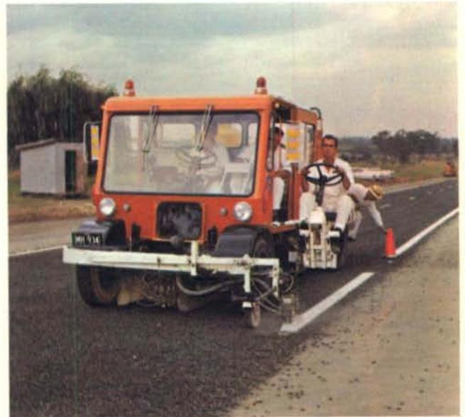
This linemarking machine was designed by the Department and manufactured at its Central Workshop, Granville.
