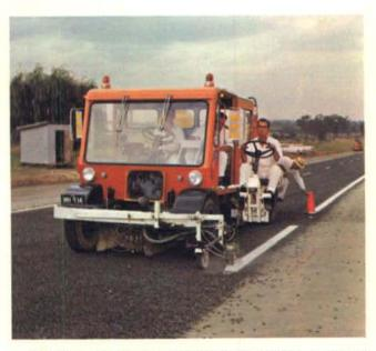
This linemarking machine was designed by the Department and manufactured at its Central Workshop, Granville.
