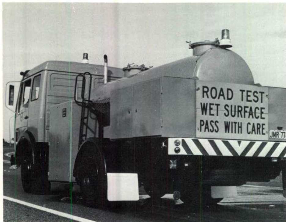
The newly acquired SCRM (Sideways-force Coefficient Routine Investigation Machine) commenced road trials in preparation for testing surface friction on all major highways radiating from Sydney.
