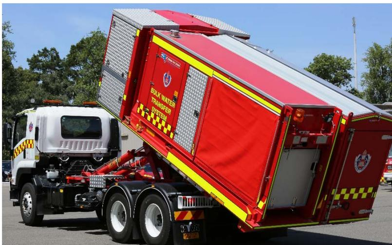
In July 2015, FRNSW took delivery of a Hytrans appliance. The Hytrans appliance can be used to supply large volumes of water (potentially around 8000 litres/minute) for firefighting at large-scale fires, across distances of up to 1.5 kilometres.
