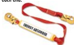
ENERGY ABSORBING WEBBING LANYARD [SA325] 2.0m with double action snaphooks at each end.
