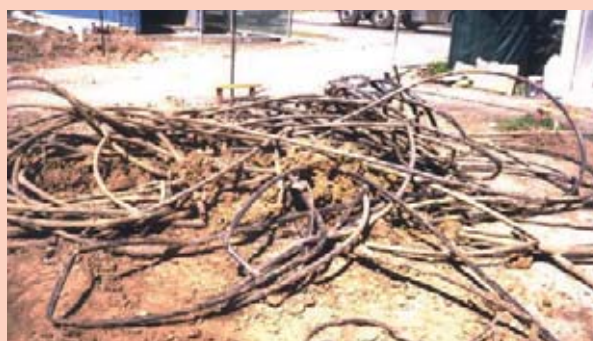
Telecommunication cable laying on a construction site, pulled out by an auger.
