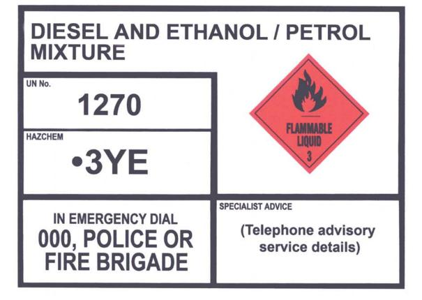
EIP for transport of petrol + diesel + ethanol and petrol mixture > 10% ethanol (different compartments)
