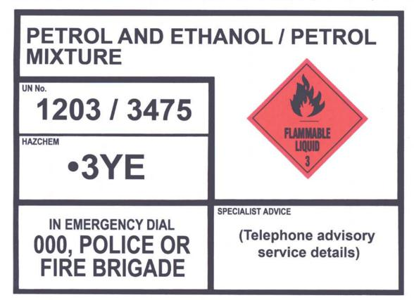
EIP for transport of diesel + ethanol and petrol mixture > 10% ethanol (different compartments)
