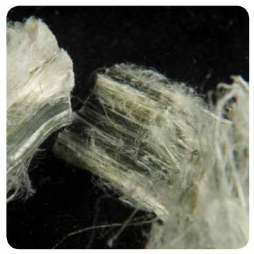
CLOSE UP IMAGE OF ASBESTOS FIBRES
