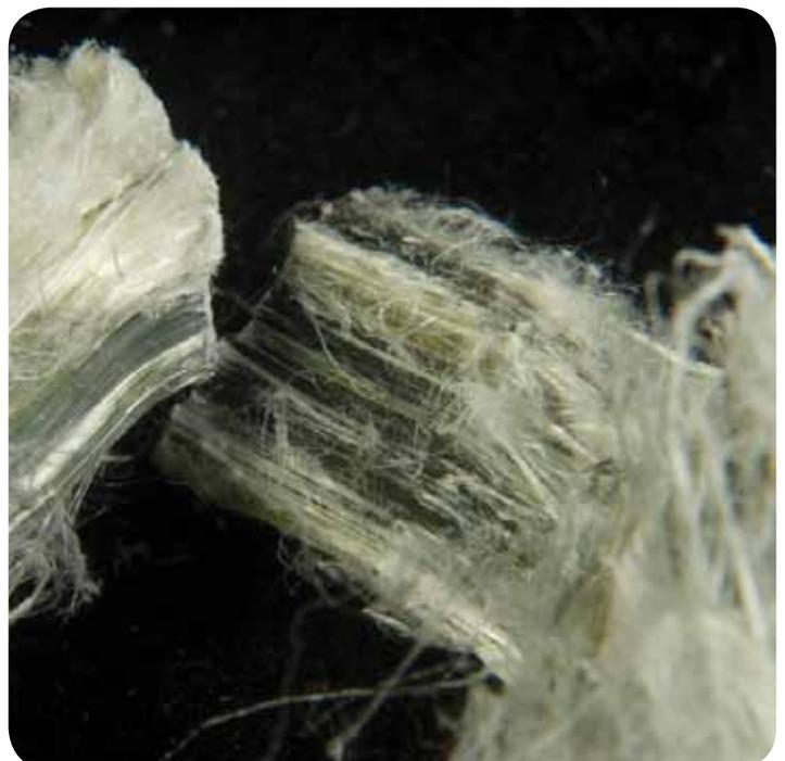
CLOSE UP IMAGE OF ASBESTOS FIBRES
