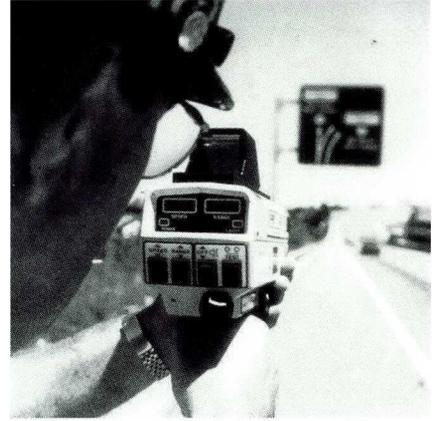
*The mobility of laser based hand held speed detectors and other new technologies, such as vehicle mounted speed cameras, make it easier for police to conduct speed deterrent operations.*
